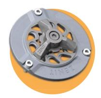
The heart of the models **GRG** is an effective, entirely redesigned **cutting device** which consists of a plate with sharp-edged holes and as a shaving, rotating triangular knife, attached to the impeller, both of which are made of **X 102 CrMo 17 KU martensitic steel.**
