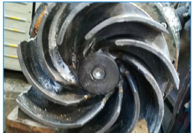
Vortex impeller with Molib-tech® coating
