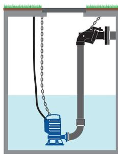
CON DISPOSITIVO DE ACOPLAMIENTO EXTERNO
