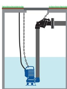
CON DISPOSITIVO DE ACOPLAMIENTO EXTERNO
