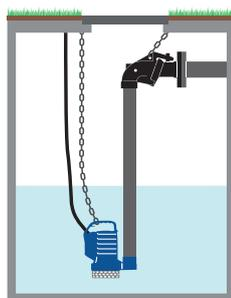
CON DISPOSITIVO DE ACOPLAMIENTO EXTERNO
